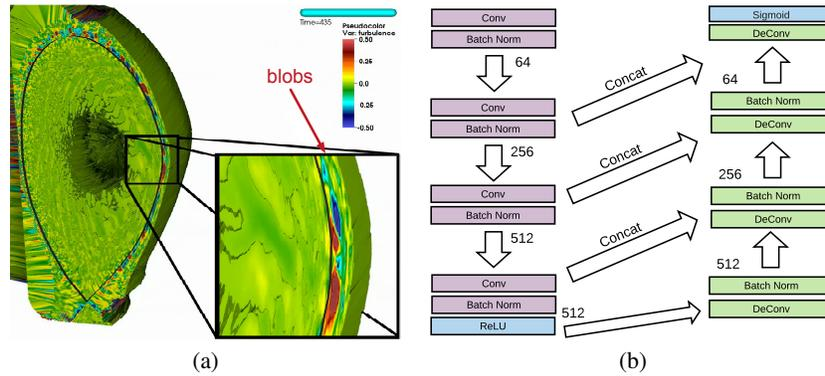
**Fig. 1.** (a) shows a zoomed view of a blob. The dark red area corresponds to the blob. (b) shows the architecture of ContourNet. Similar to U-Net, ContourNet has two phases. However, there is no change of the image size. The numbers in the figure show the number of channels after a given batch normalization.
